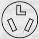
3-wire receptacle (10-30R)
